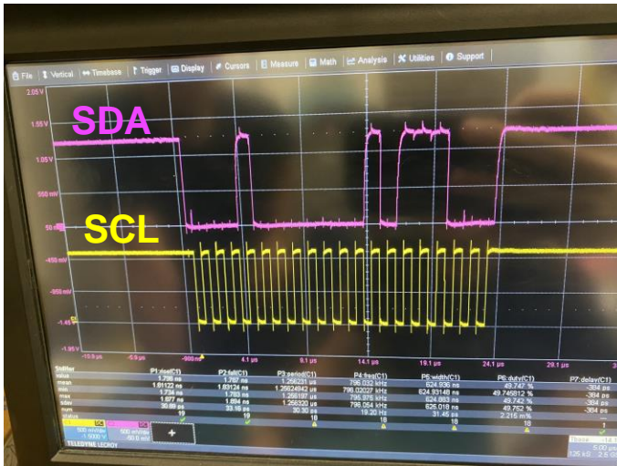
A successful I2C transaction between two front end ASIC
