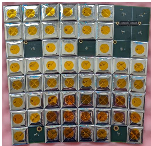
TB3 board 1 equipped with moulded tiles Batch 1 with pre-series 4mm 2 SiPMs
