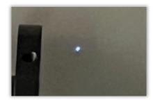
SFG of 1550 nm with 515 nm (387 nm)
