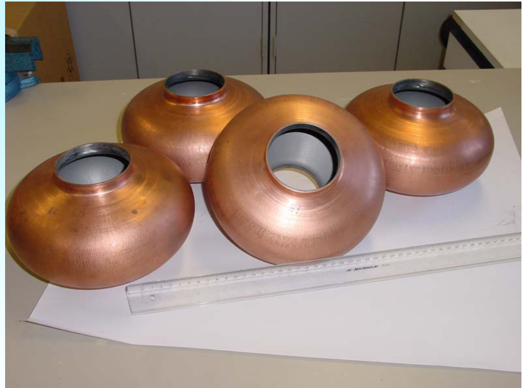
Single cell cavities produced from Nb/ Cu0.15%Zr clad tube
