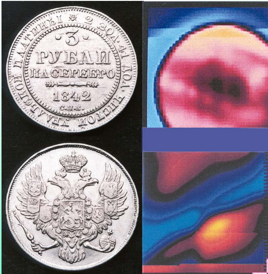
SQUID-test on a russian coin made of raw-platin in powder metallurgy with PtIrFe-phases
