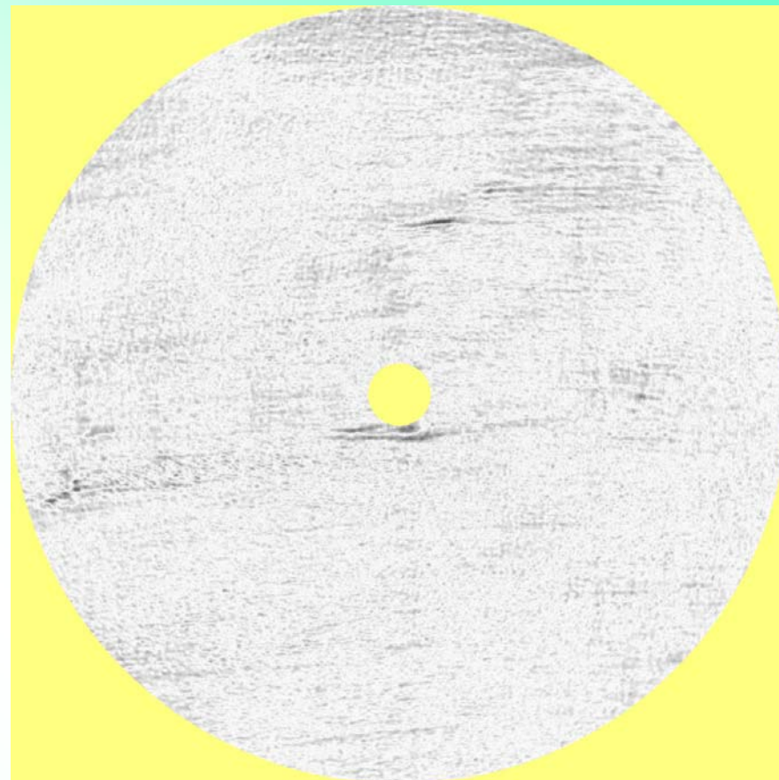
Eddy Current image of the NC-1357-400 Nb-sheet
