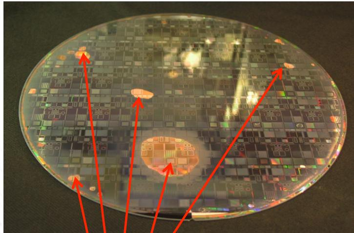
Damages on the wafer & Close up photographs
