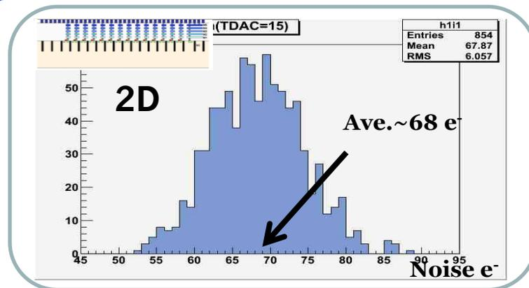
Slightly higher noise of the 3D chip wrt. 2D
