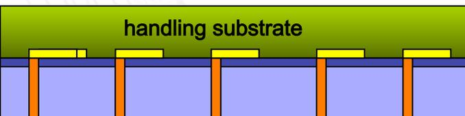
Bonding to handling substrate, thinning to 50  $\mu\text{m}$
