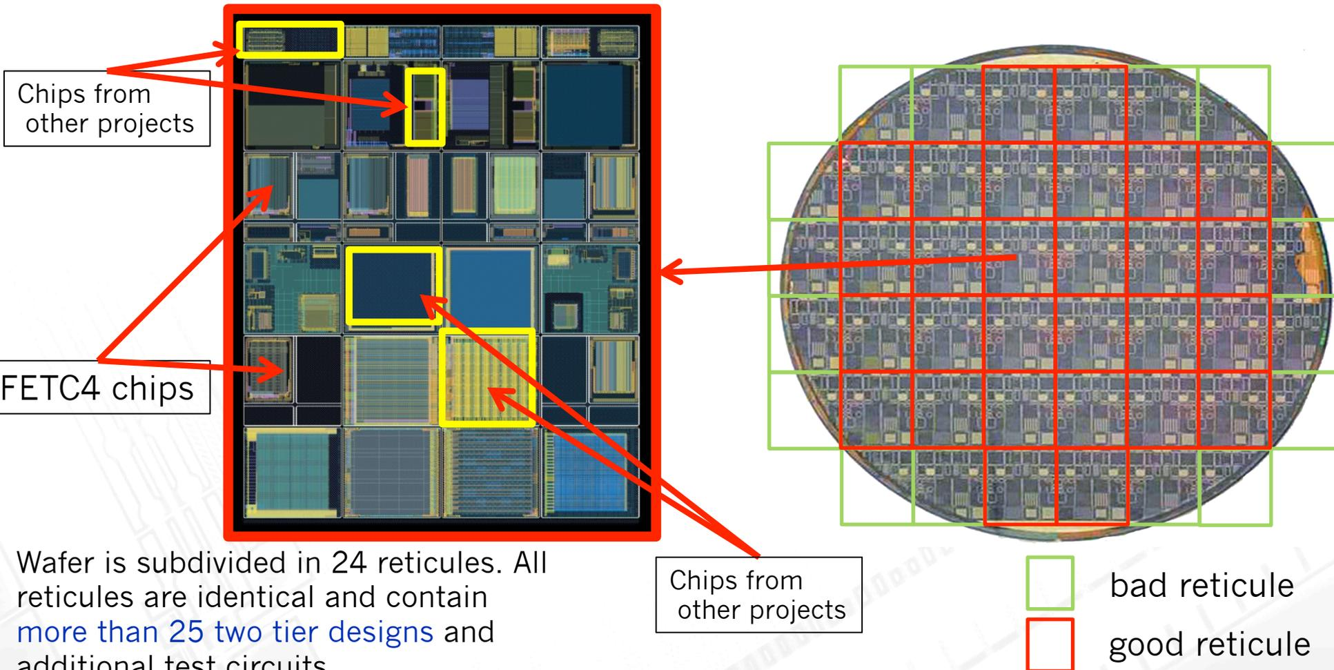
Wafer is subdivided in 24 reticules. All reticules are identical and contain **more than 25 two tier designs** and additional test circuits.
