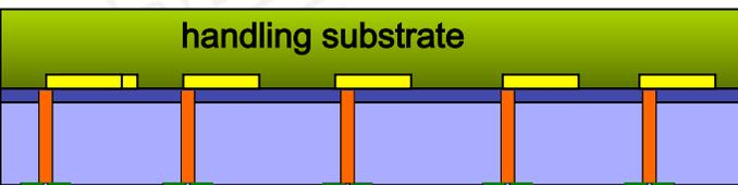
Exposure of W in TSV and Alu spattering for creation of pads on the back-side
