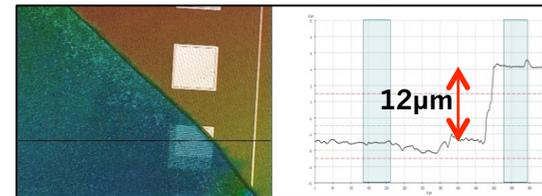
near damage. Level shift  $\sim 12\mu\text{m}$  = thinned layer thickness
