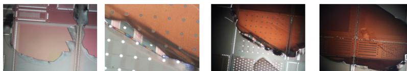
Bad mechanical connection between tiers → top tier removal during thinning process
