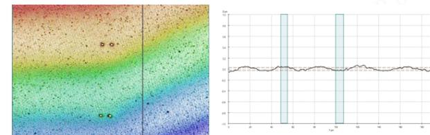
@ no damage. Level variation  $\sim 30\text{nm}$
