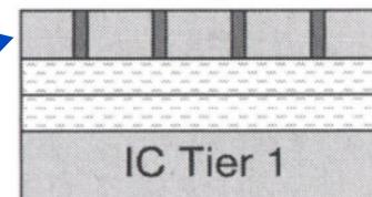
Wafers are placed one on top of another and aligned to match Bond interfaces of both tiers.
