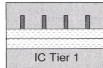
3. wafer thinning & backside processing
