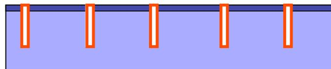
TSV Isolation with SACVD  $\text{SiO}_2 \sim 300 \text{ nm}$
