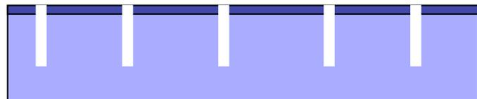
SACVD Pad Planarization, TSV Litho, Etching with Bosch process, cross section  $\sim 4 \times 10 \text{ mm}^2$ , depth=60  $\mu\text{m}$
