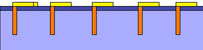
Electroplating of Cu on the front side
