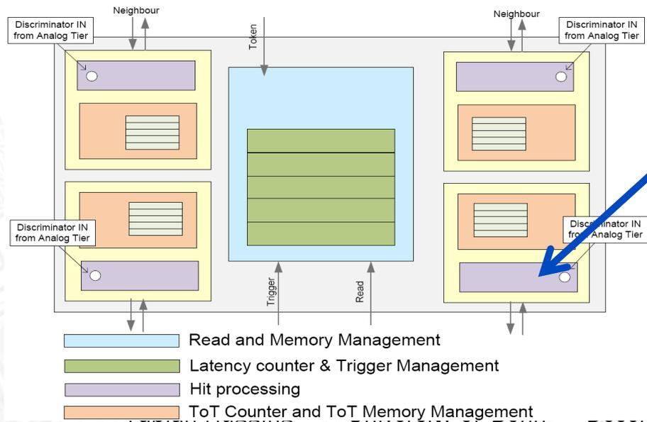
Analog pixel chain and 4-pixel Region derived from FE-14
