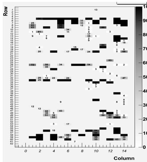
Bad electrical & mechanical connection due to misalignment of the tiers.
