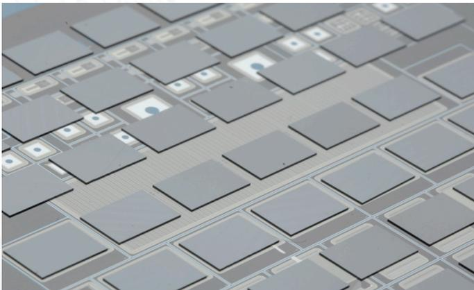
FE-13 chips (mostly not electrically functioning) used to improve the pressure homogeneity on the wafer during the SLID interconnection
