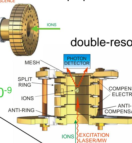
in-trap spectroscopy (SPECTRAP)
