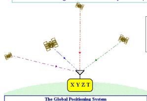
A receiver deduces its TXYZ-positions from radio signals emitted by at least four satellites
