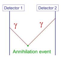
Collecting measurements of the two detectors allows one to deduce the positions in space <u>and</u> time of the event
