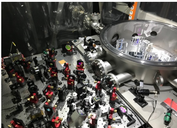
Central optics breadboard of the ALPS II experiment
