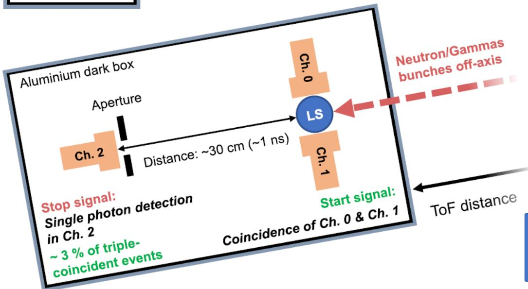
In both experiments we distinguish neutron interactions from beam correlated gammas by time-of-flight (ToF) measurements!
