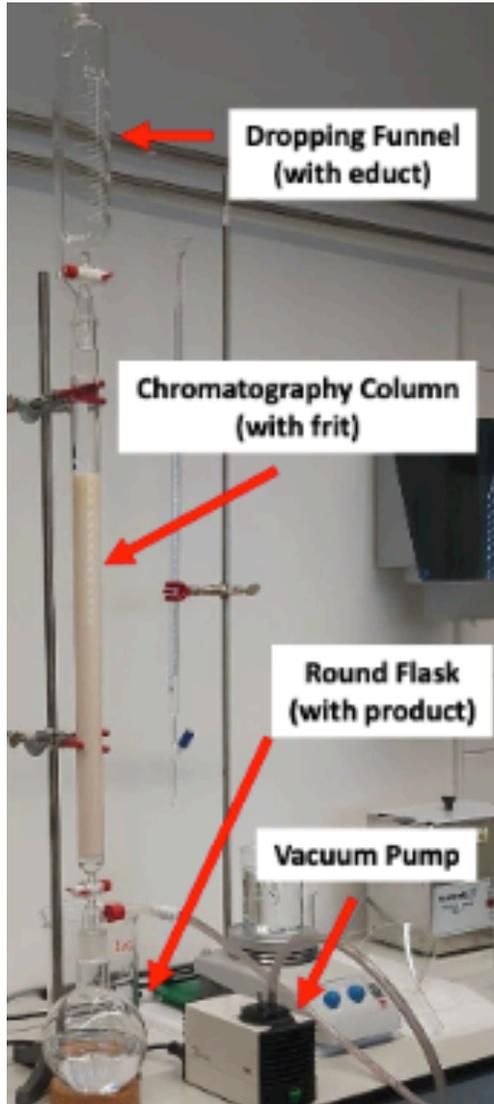
Long and thin  $\text{Al}_2\text{O}_3$  Colum (basic alumina of activity Super-I
