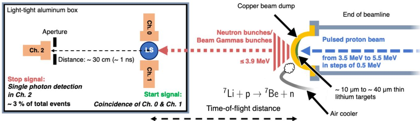
Neutron production at the CN Accelerator:
