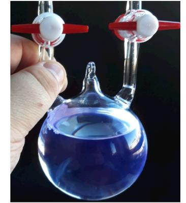
Sphere with Target Medium for the PSD-Experiment
