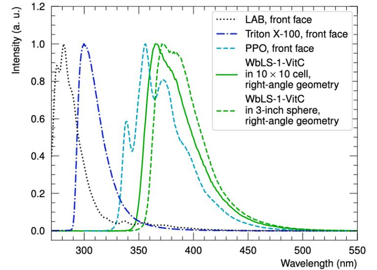
Emission Spectra of WbLS and its Components
