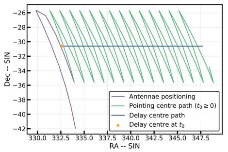
Antenna pointing and delay setup for MeerKAT scans: array scans back and forth in azimuth at fixed altitude, while the Earth rotates new sky into view
