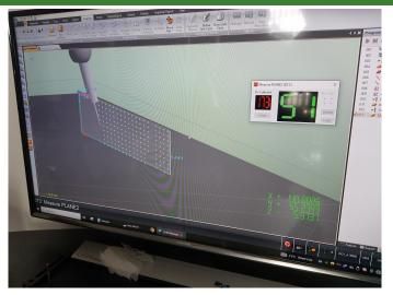
$\bullet~\sim 250 = 10 \times 25$  XY points on each side, starting 2.5mm from the edge
