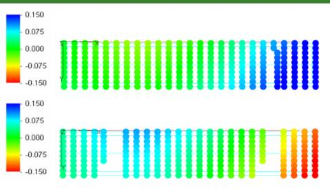
• bending > 150  $\mu\text{m},$  for large X plus some "wave" in the middle , $\sim$  75  $\mu\text{m}$
