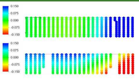
• the worst plate, planes not parallel, edge cutting due to non uniform grinding ?
