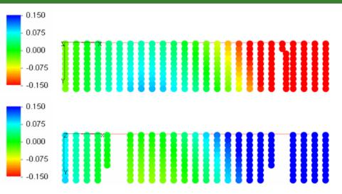
• big bending, > 150  $\mu m,$  for large X plus some "wave" in the middle, ,~ 75  $\mu m$
