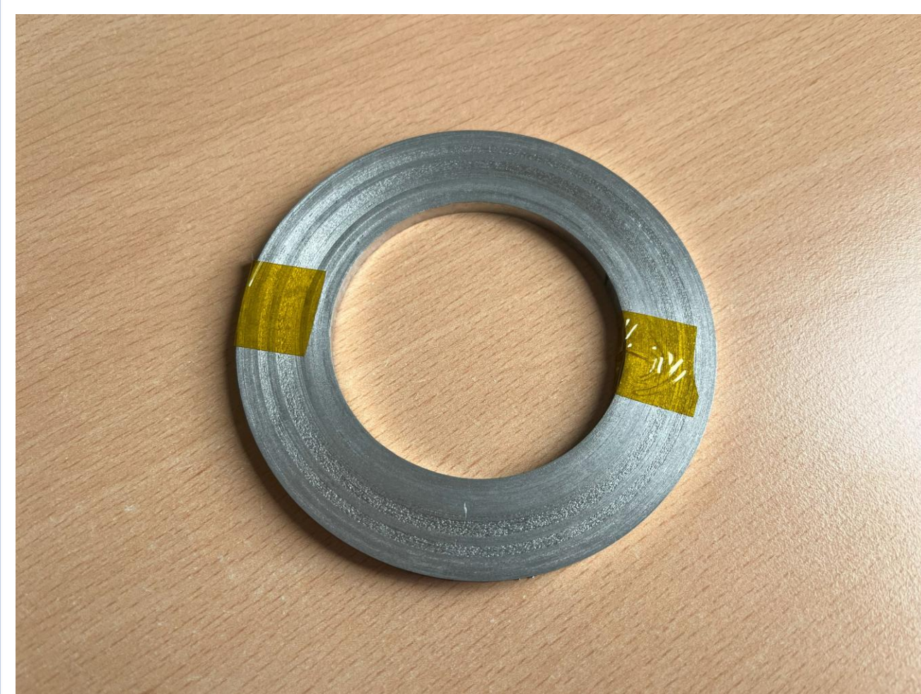
Soldered Pancake, 276 turns (courtesy of M. A. Hafiz and G. Scarantino)
