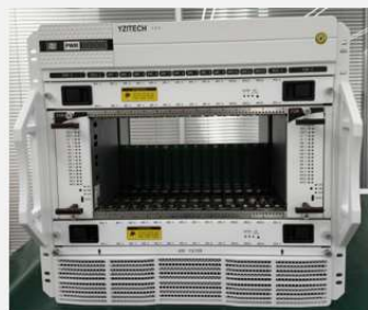
MTCA Chassis + Power(10U) Supports 12 AMCs, 2 MCHs, and 2 PDMs.
