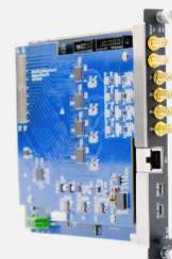
AMC DAQ card Zynq UltraScale , 4CH500M sampling rate, 6GB DDR4
