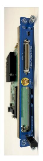
AMC Module, ZYNQ 7000 Designed by DESY, Built under license by D-TACQ.
