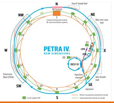
The new PETRA IV accelerator will replace PETRA III with an **ultra low** emittance ring (20 pm) adding new experimental halls in two more octants.
