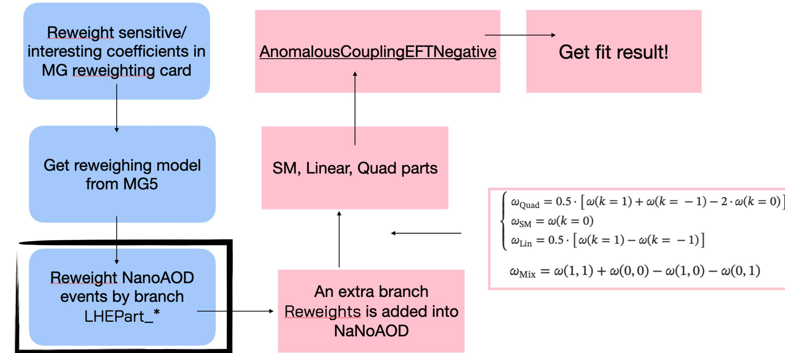
It's doing a mapping from a PDG list got from MG5 production to NanoAOD LHEPart
