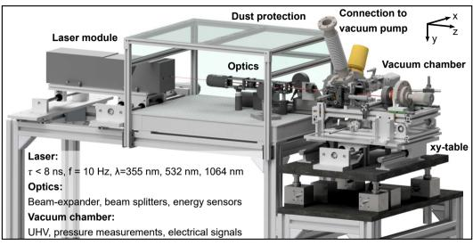
Setup created in last project ⇒ Point and area polishing of samples under vacuum and defined atmospheres
