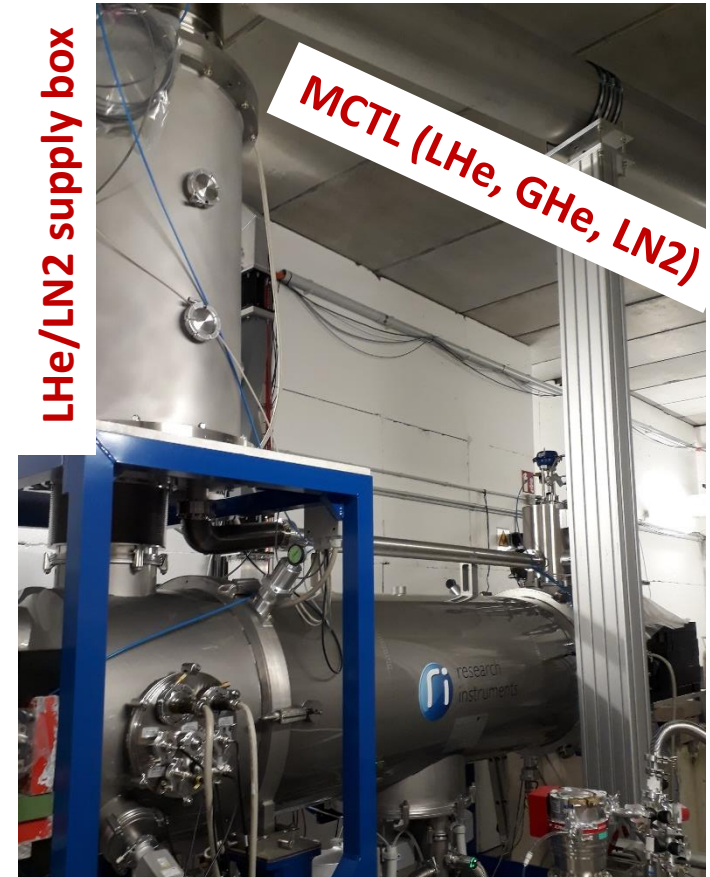
Cryomodule (2 XFEL Cavities @ 12.5 MV/m)
