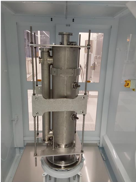
HPR: (TESLA recipe) each cell rinsed for 5 min (18x)
