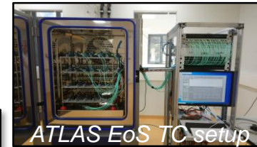
ATLAS hybrid burn-in setup
