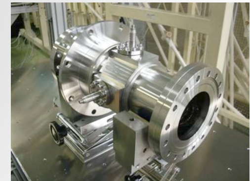
Fabricated L-band BPM prototype. S. Jang, H. Hayano et al., Development of L-band cavity BPM for STF, IPAC19
