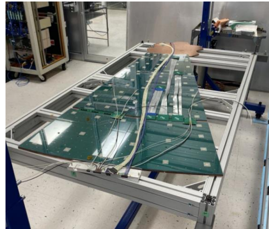
20° mixed cassette mechanical mockup
