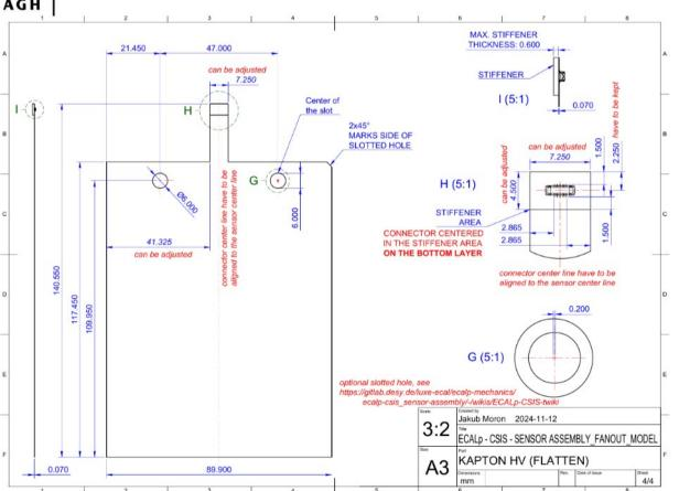
Flatten ("production mode") drawing of the HV kapton
