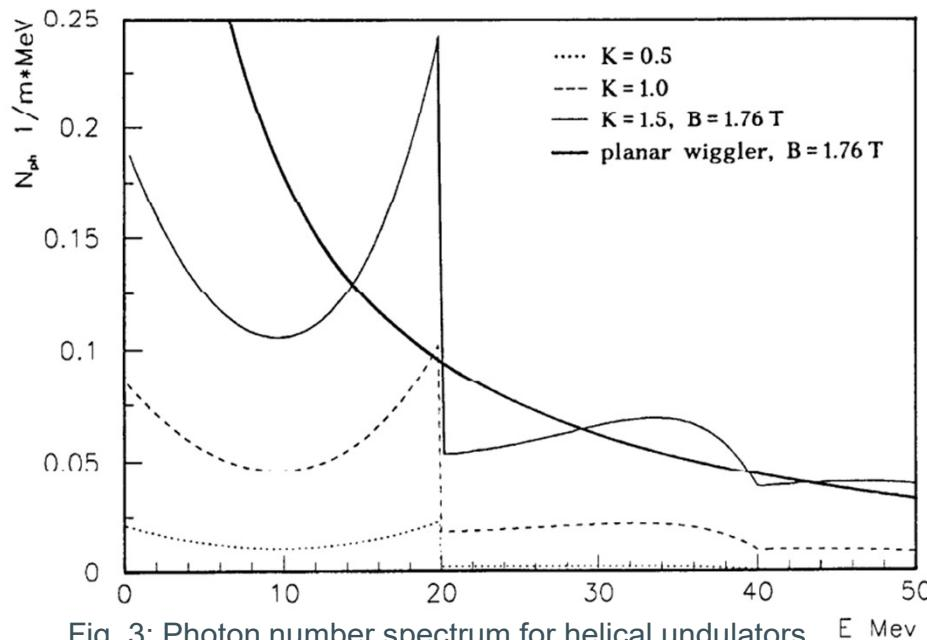
Fig. 3: Photon number spectrum for helical undulators
