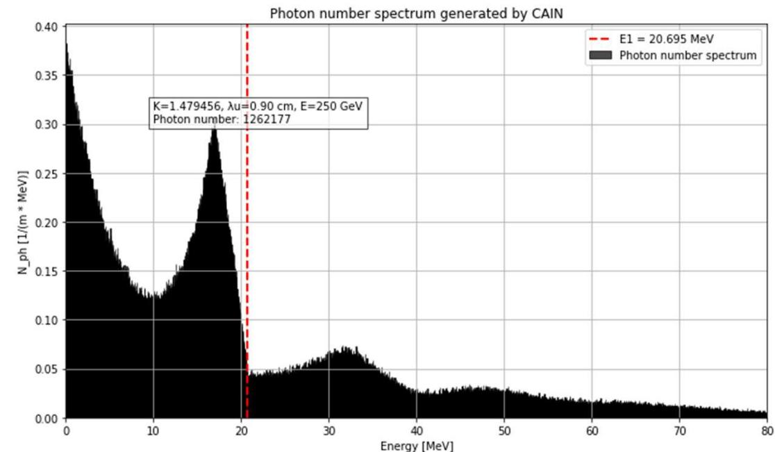
Fig. 4: Photon number spectrum by CAIN
