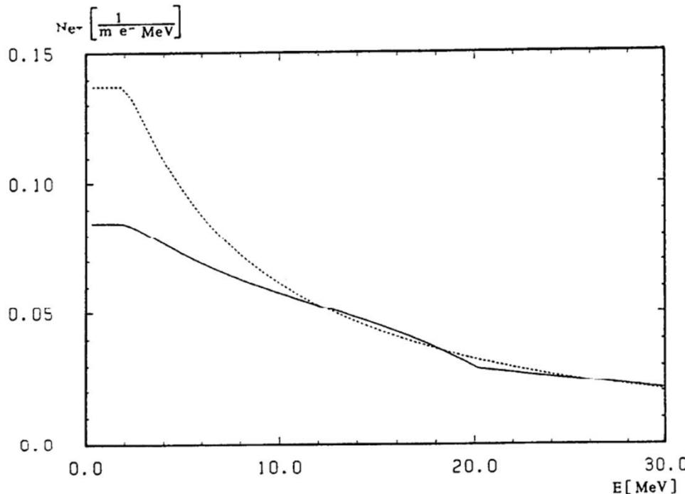
Fig. 5: Estimated positron spectrum for helical undulator
