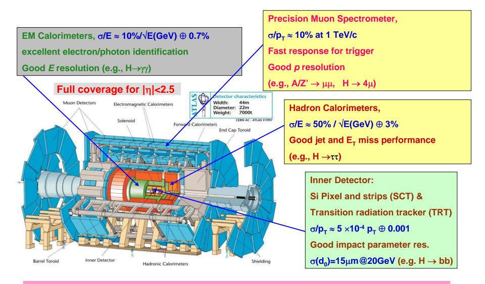
Magnets: solenoid (Inner Detector) 2T, air-core toroids (Muon Spectrometer) ~0.5T
