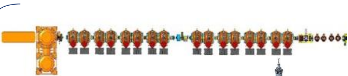
Low-Energy Cooler, IR02 - 17 197 QWR NCRF, 4 591 NCRF, 1 24 MHz NCRF, And 1 591 MHz Deflecting Cavity
