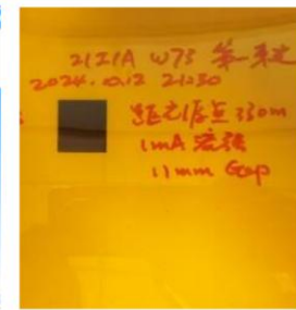
Oct. 12, 2024 the SR X-ray emitted from the R21 wiggler was successfully transmitted to the end station.
