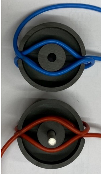
Fig. 2: Implemented coils in this Letter. (a) Coils, with a diameter of 6.6 cm. (b) Multi-layer self-resonant structure (MSRS) internal architecture, with an integrated capacitance and thin foil layers [29].
