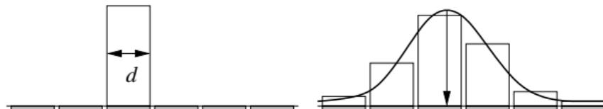
Charge-sharing for a good spatial resolution using pad-readout
