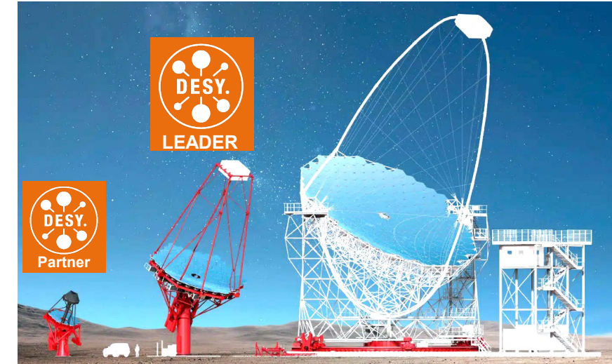
SST, \varnothing 4.3 m MST, \varnothing 11.5 m LST, \varnothing 23 m
