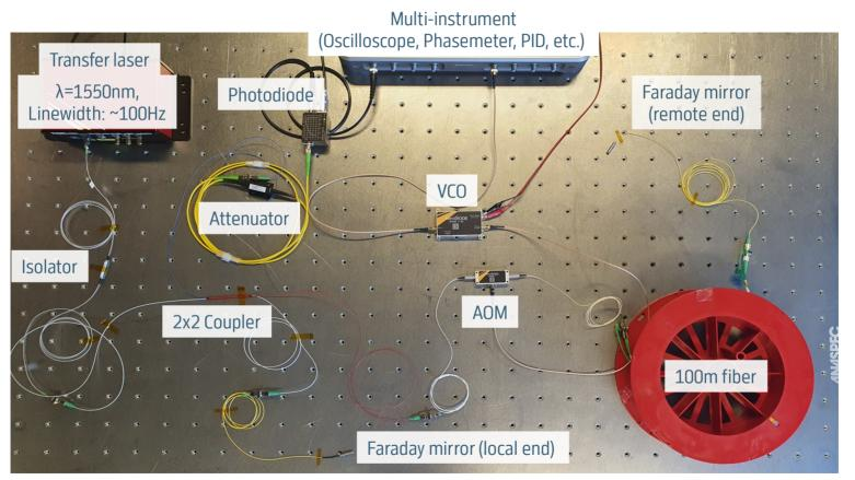
Fiber Michelson-interferometer uses RF beat note to identify & correct for phase noise
