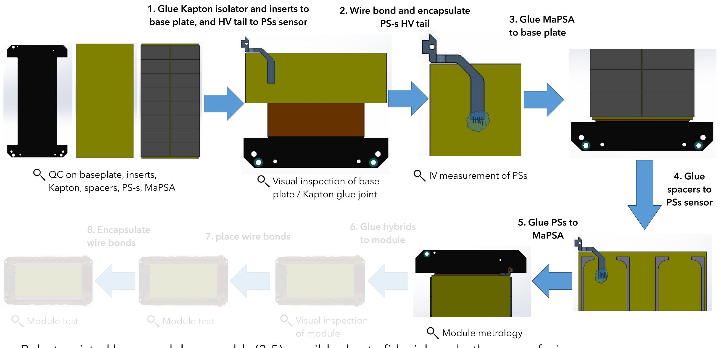
Robot assisted bare module assembly (3-5) possible due to fiducials on both sensors facing upwards
