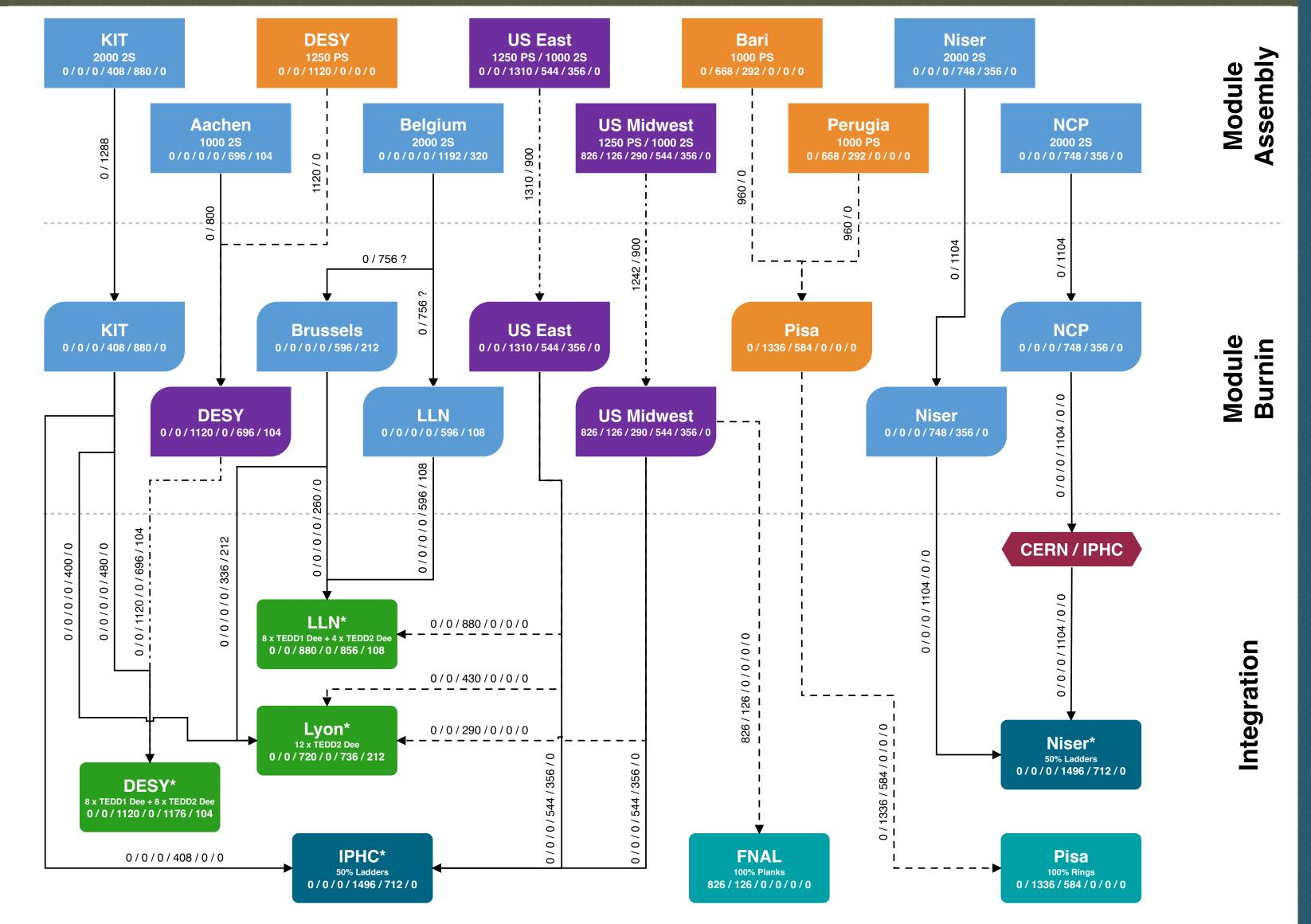
Module type list: 1.6 mm PS / 2.6 mm PS / 4.0 mm PS / 1.8 mm 2S 5CP / 1.8 mm 2S 6CP / 4.0 mm 2S
