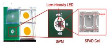
SiPMs consists of thousands of single photon avalanche diodes (SPAD) working in Geiger-Mode
