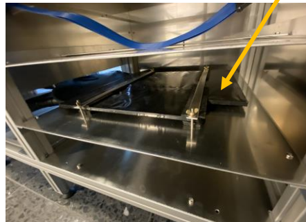
Trigger scintillator (size: ~45 x 45 cm)
