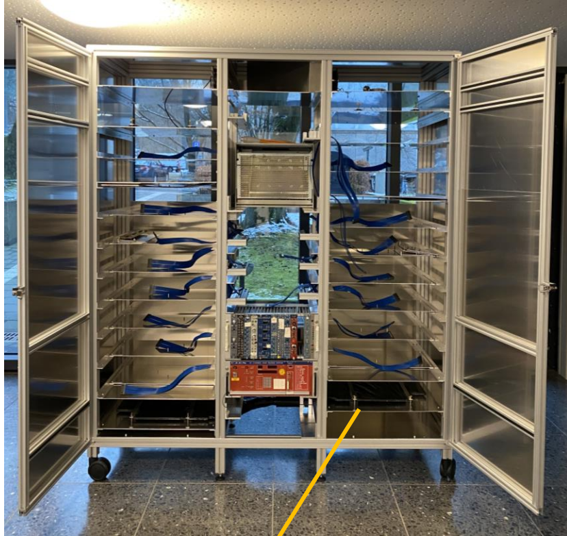
Trigger scintillator (size: ~45 x 45 cm)
