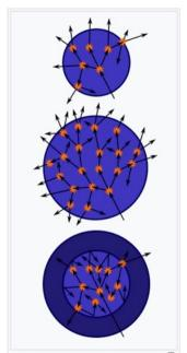
Top: A sphere of fissile material is too small to allow the chain reaction to become self-sustaining as neutrons generated by fissions can too easily escape.
