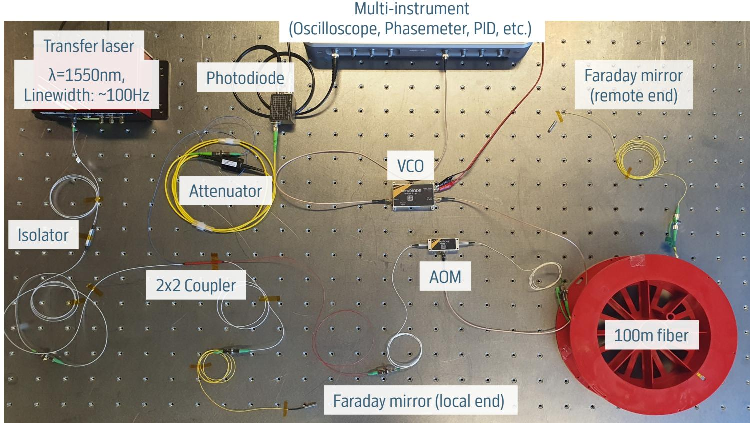
Fiber Michelson-interferometer uses RF beat note to identify & correct for phase noise
