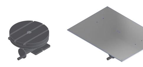
Additional plate to host ECAL-P on rotary table
