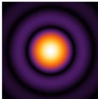
A central peak surrounded by concentric rings of alternating high and low intensity, characteristic of an Airy disk. |
