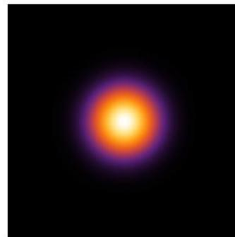
A circular Gaussian beam profile showing a central bright spot (peak) fading into a dark background. |
