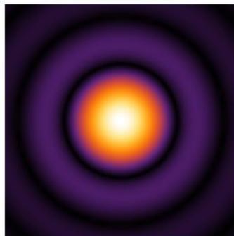
An Airy disk profile showing concentric rings of intensity centered on a bright peak. |
