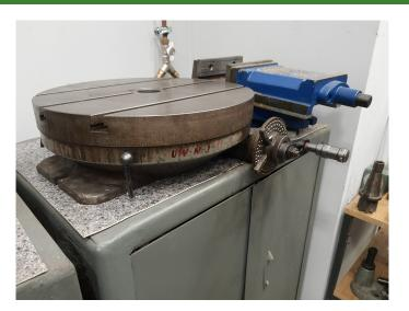
• load > 50 kg, resolution  $\sim$  0.5 [deg] (manual wrt the scale), better with laser pointer wrt the mirror  $\rightarrow$  work in progress
