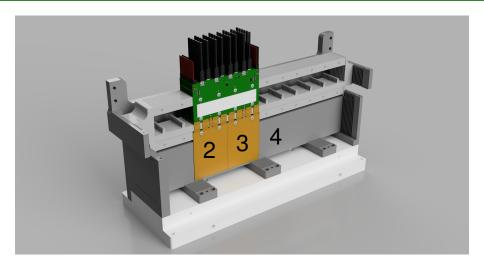
Sensors at positions (2,3) to be shifted to (3,4) at the center on rotation axis (accepted by Jakub)
