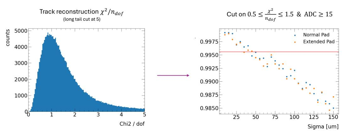
Extended pad – added  $2\mu m$  on each side to roughly account for angles  $\rightarrow$  no significant difference
