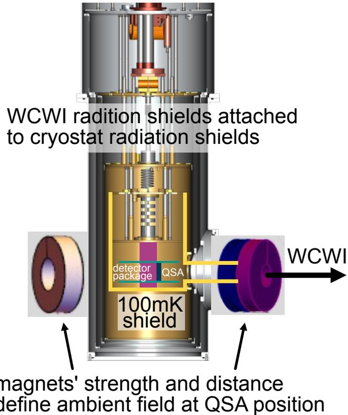
a temperature stage should ideally have a direct line-of-sight to the next higher temperature stage
