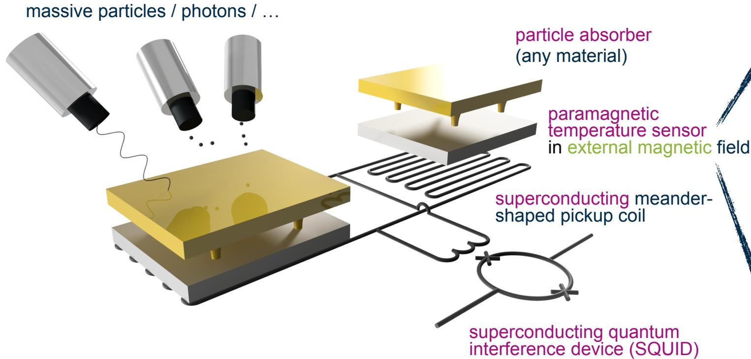
magnetization of a paramagnetic material
