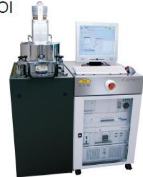
Direct and adhesive (temporary) bonding: EVG501
