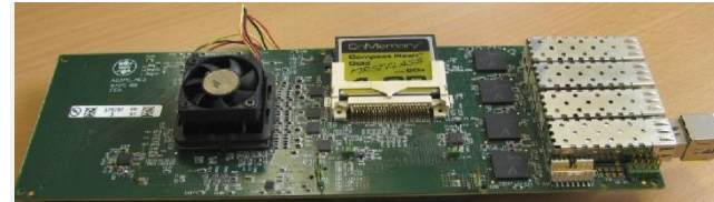
Old Mezzanine shared with 1 st -gen. AGIPD and LAMBDA systems
