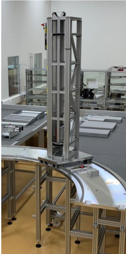
Insertion tower on tower platform with rail system
