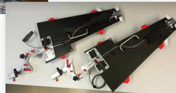
Petal hands for lifting of petal (FL and BL variant) – designed against bending frame
