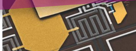
MMC detector: world record in energy resolution of 1 eV
