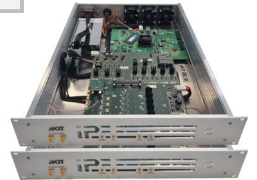
ECHO readout system for 800 MMCs
