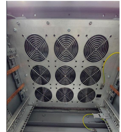
Cooling with EMI fan top cover and 9 fans
