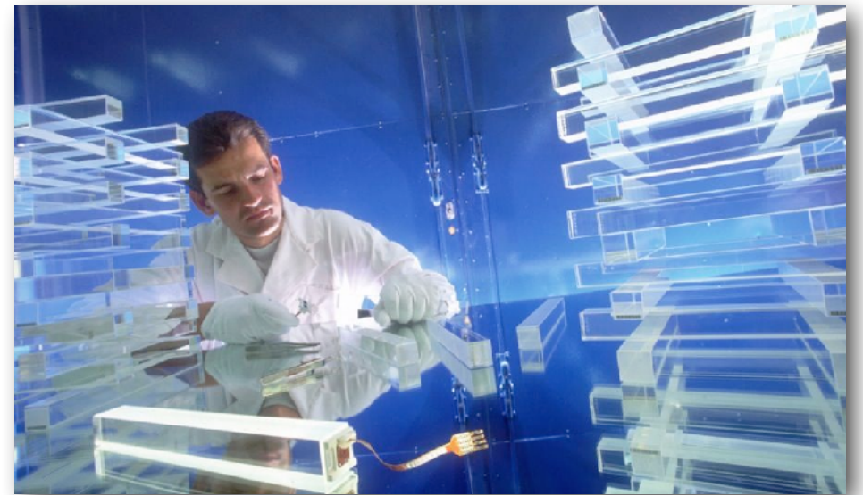
CMS Lead tungsten crystals, each 1.5kg (CERN)
