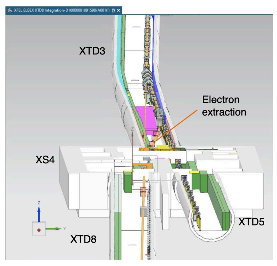
First concept of double-bend ELBEX extraction beamline, to be optimized
