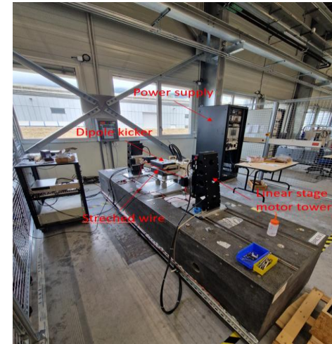
Test bench with a dipole kicker.
