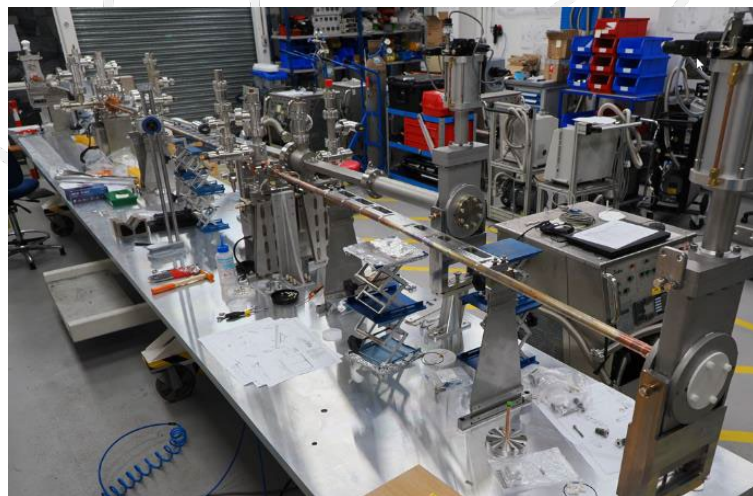
Full prototype girder vacuum vessel string
