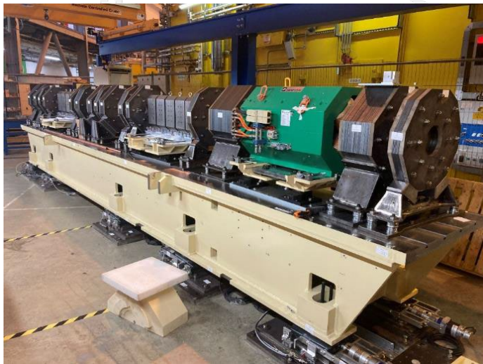
Prototype girder with dummy magnets for vibration and alignment tests
