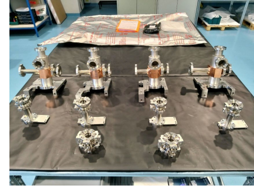
Pre-series girder fabrications
